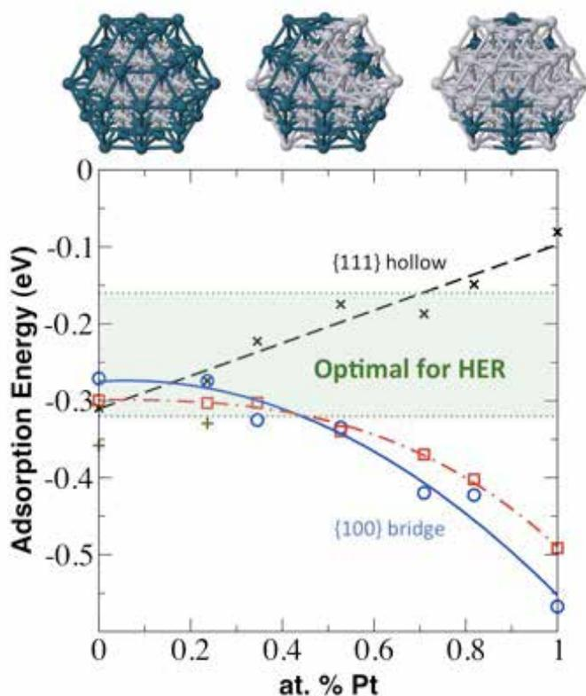
Figure 3: H-adsorption energy of Pd-Pt nanoalloy groundstates as a function of composition. Adsorption trends for {111} hollow, {100} bridge and edge-bridge sites are denoted by crosses, open circles and squares respectively. Lines are best-fit curves. Adsorption energies in the region shaded green are optimal for the hydrogen evolution reaction.
