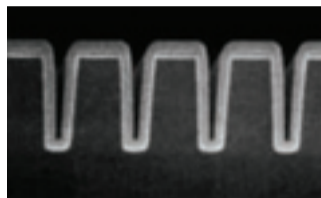
Cross-sectional SEM image for 300nm Al 2 O 3 film deposited using ALD technology
