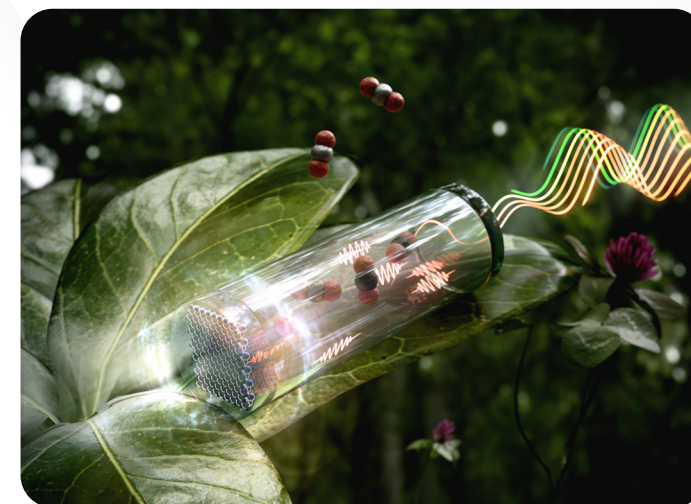
▲ Miniaturised NDIR CO 2 gas sensor (4 cm long, 0.1 cm diameter) based on 20% ScAlN pyroelectric detector
