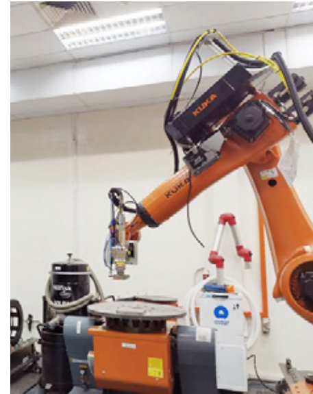
▲ SIMTech robotic hybrid laser-aided additive manufacturing system.
