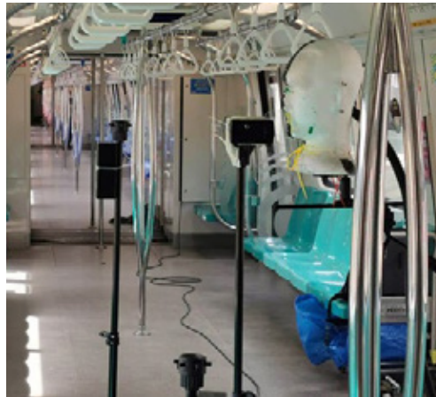
▲ Experimental design of smoke spread in a moving train cabin.
