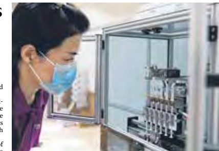
Nurse Nellie Tan, 47, with the Automated Vaccine Inoculation Dispenser system, which weighs less than 25kg and can fill six syringes in under five minutes. It has been deployed at seven vaccination centres islandwide. ST PHOTO: NG SOR LUAN
