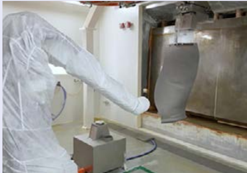
A robotic spray system for fan blades of aircraft engines (Credit: Rolls-Royce)
