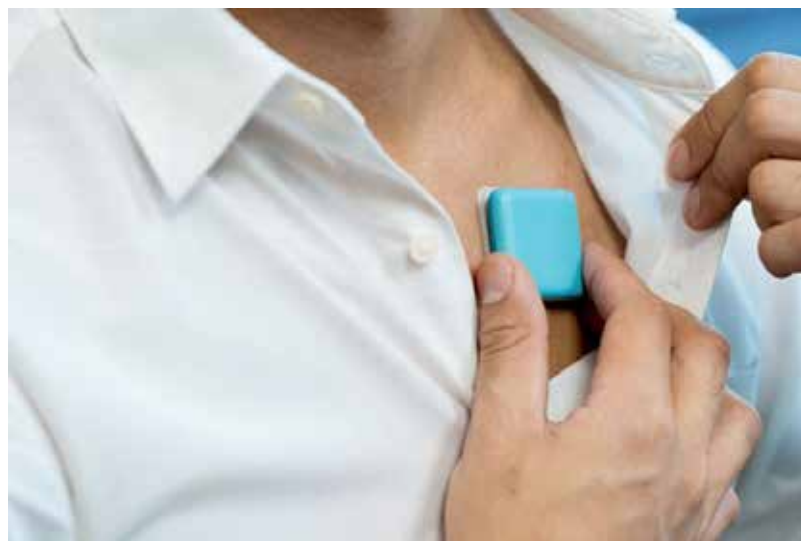
Local medical technology start-up Respiree's wearable device which is used to measure vital parameters such as respiratory rate or blood oxygen levels.
