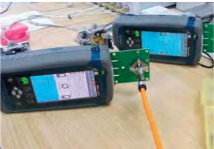
Comparative testing with Psiber’s handheld network analyzers in NMC’s lab
