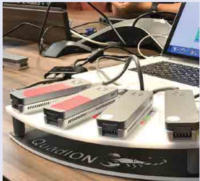
These are portable DNA sequencing devices created by Oxford Nanopore Technologies, called MinION.
