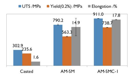
Tensile properties of all AM-made soft magnets (SM) tested by MTS mechanical tester. The AM-made soft magnetic composites (SMC) show both higher tensile strength and ductility than conventional casted magnet.
