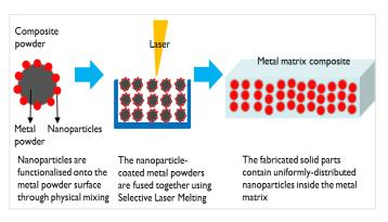
Schematic diagram illustrating the methodology for making metal matrix composites using Selective Laser Melting.
