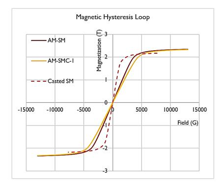
Magnetic hysteresis loops of all AM-made soft magnetic materials tested by Vibrating Sample Magnetometer (VSM) at room temperature, show strong saturation magnetisations.
