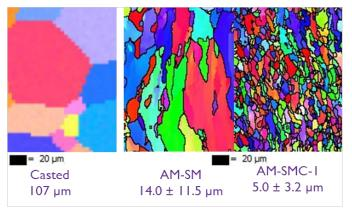
Microstructures of all AM-made soft magnetic materials measured by Field Emission Scanning Electron Microscopy-Electron Backscatter Diffraction (FESEM-EBSD). AM-made soft magnets (SMs) show more refined grain structure than conventional casted magnets. Nano particle-reinforced soft magnetic composites (SMC-I) show significantly refined grain sizes.
