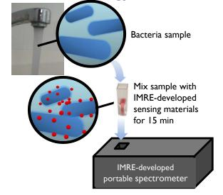
Bacteria detection using the IMRE nanomaterials-based sensor and IMRE-developed portable spectrometer
