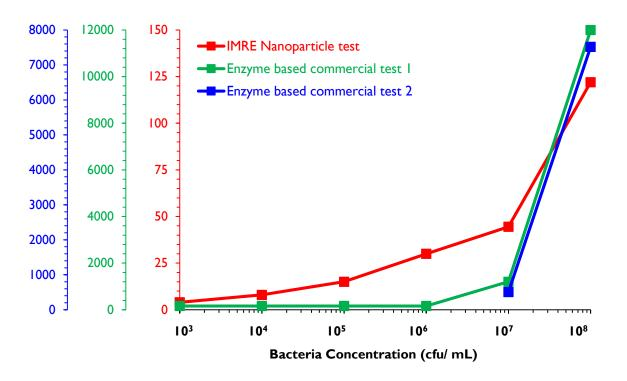
The increase in sensing signal is proportional to live bacteria concentration and helps to differentiate between dead and live bacteria.
