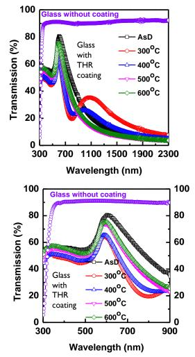
The transparency of the THR at 600nm is  $\sim$ 81% for Asdeposited THR. After annealing at a temperature of 600°C, the transparency of the THR is changed only very slightly.
