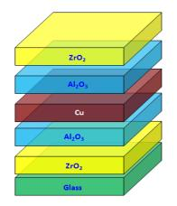
A schematic diagram of the structure of the THR applied on glass. The structure includes copper (Cu) for heat reflection, zirconium oxide ( $ZrO_2$ ) for adhesive, antireflection and anti-scratch properties and aluminum oxide ( $AI_2O_3$ ) to act as an oxygen diffusion barrier and to enhance durability.
