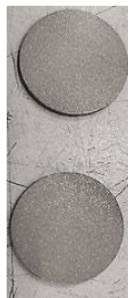
Porous steel with controlled pore size and porosity level
