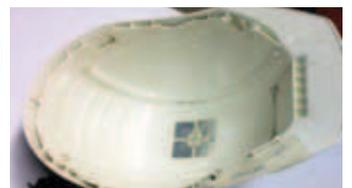
RFID Tag attached non-disruptively onto the safety helmet
