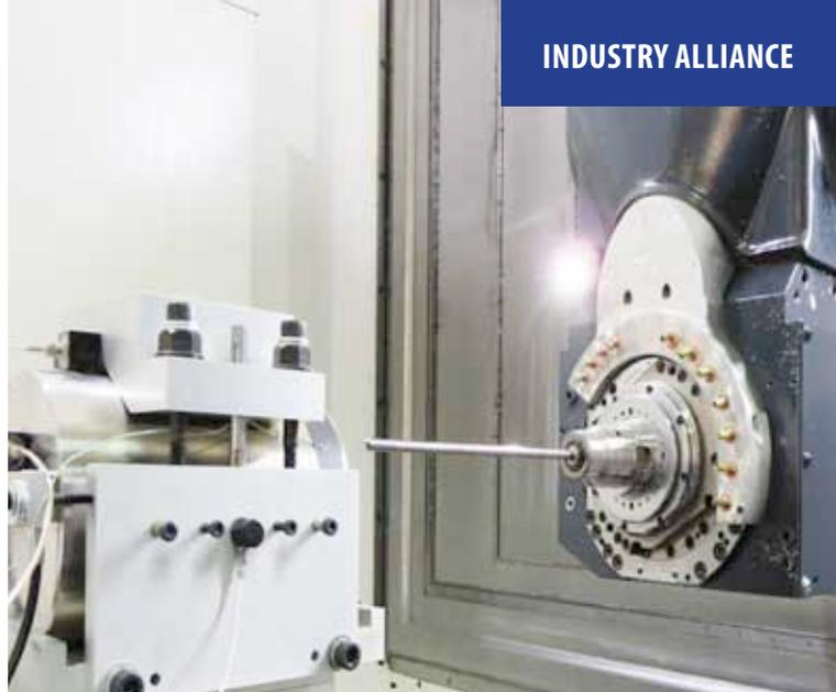
SIMTech has pioneered an evaluation, comparison, and validation method to produce deep, straight holes in a variety of materials for downhole drill pipes to enable Oil & Gas exploration venture into greater depths and harsher environments. With assistance from SPRING Singapore, SIMTech launched an initiative under its CIP scheme to equip companies in the Oil & Gas sector with effective tooling, preparation methods, and drilling parameters.
