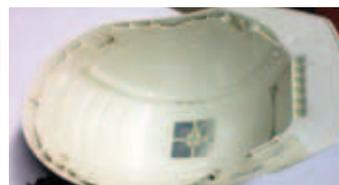
RFID Tag attached non-disruptively onto the safety helmet
