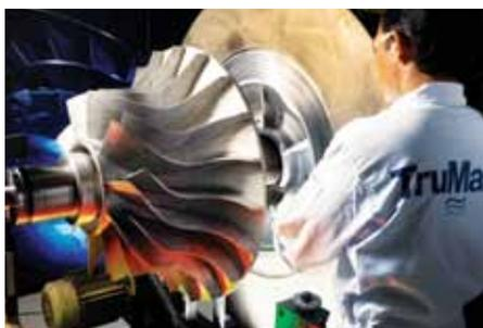
marine, a specialist in maintenance, repair and overhaul of turbochargers for the marine, offshore, power plant and locomotive applications. Suitable for repairing most of the turbocharger components, the system and process improved productivity and property significantly. This technology is commercialised for the repair of turbocharger components.
