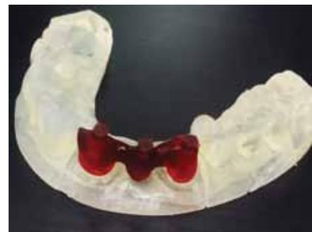
Arising from this programme, SIMTech is currently working with several dental labs on technology optimisation for 3D printing of patient specific wax-ups, dental models and ceramic crowns and bridges. By combining stereolithography with investment casting, customised dental crowns and bridges are produced in a faster and more efficient way.
