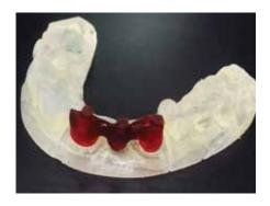
Arising from this programme, SIMTech is currently working with several dental labs on technology optimisation for 3D printing of patient specific waxups, dental models and ceramic crowns and bridges. By combining stereolithography with investment casting, customised dental crowns and bridges are produced in a faster and more efficient way.
