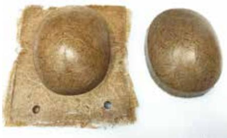
To do this, SIMTech examined the potential use of natural fibre composites in ear cups and ear plugs, carried out processing of composite preform (prepreg), manufacturing process for the ear cups and investigation of acoustic performance. The composite ear cups were manufactured by incorporating
