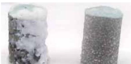
Comparison between bare (left) and coated (right) magnesium samples after 28 days immersion in simulated body fluid solution indicating severe corrosion and pitting of the unprotected metal while only moderated corrosion is seen on the coated part
