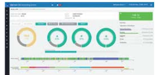
machine downtime and maximise machine utilisation. By monitoring and analysing the performance of all of JEP's 90 machines, the OEEMS improves company machine utilisation by close to 30 per cent and achieves 15 per cent increase in yield.
