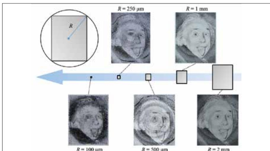
Scaling down of the machined grayscale images on metal surfaces
