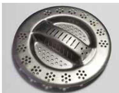
Figure 1: Development of metal “chokeless” strainer design and processing steps through simulation modelling (left) and stamping trials – a stainless steel strainer prototype with opening features optimised for stamping process steps (right)
