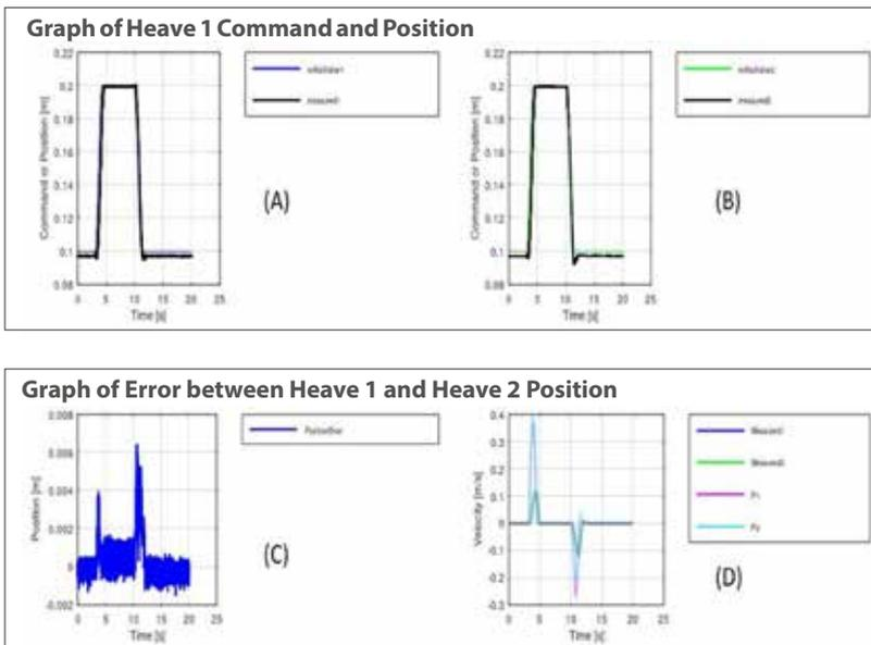
Figure 1 (A) The position(black) and command(blue) of hydraulic cylinder 1. (B) The position (black) and command(green) of hydraulic cylinder 2. (C) The position error between hydraulic cylinder 1 and hydraulic cylinder 2. (D) Measured velocity of hydraulic cylinder 1 and 2
