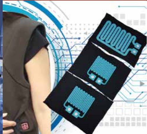
Printing of micro heaters (left), Printed heater (right)
