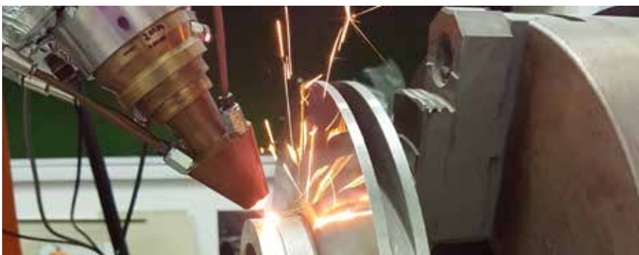
Cladding restores the original dimensions of impellar blades due to wear and tear after heavy usage over time
