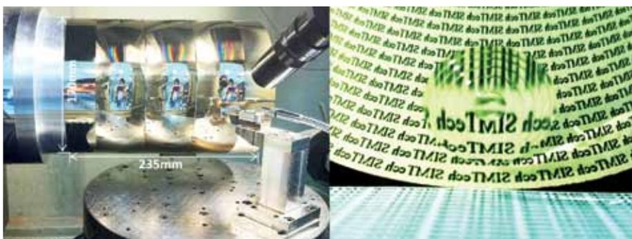
Machined linear/radial Fresnel lens roller moulds
