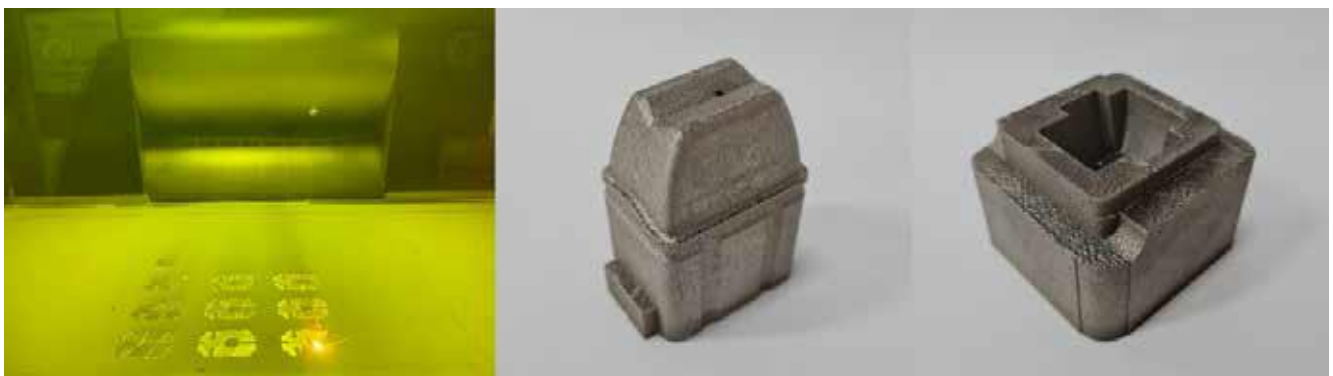
Figure 15 Ready demonstrator of a cavity and insert build in DMP Flex 350 in full-built.
