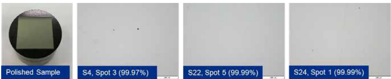
Figure 12 Optical microscope images of an LT30 polished sample at 100x magnification.
