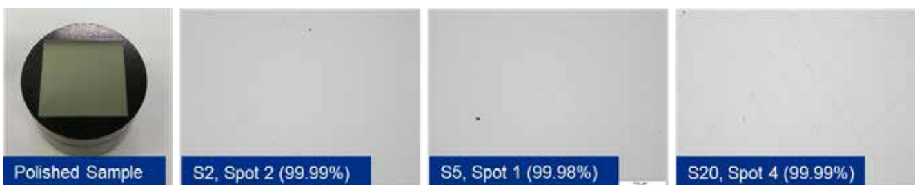
Figure 13 Optical microscope images of an LT60 polished sample at 100x magnification.
