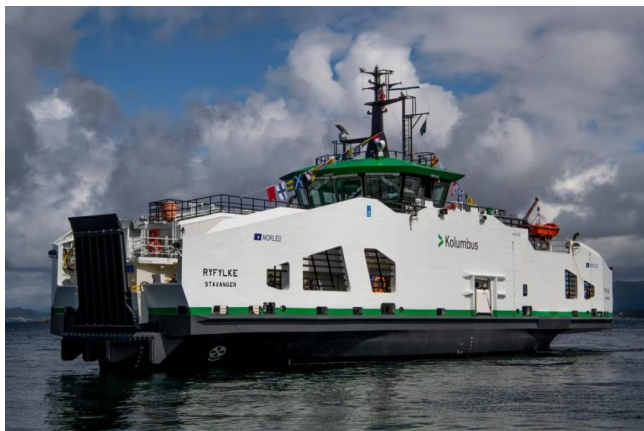
NORLED Ryfylke - First battery powered vessel to operate a full day without shore charging.
