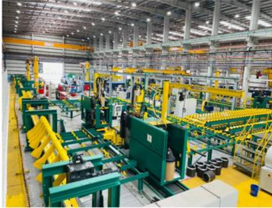
Robotic automation for visual weld inspection
