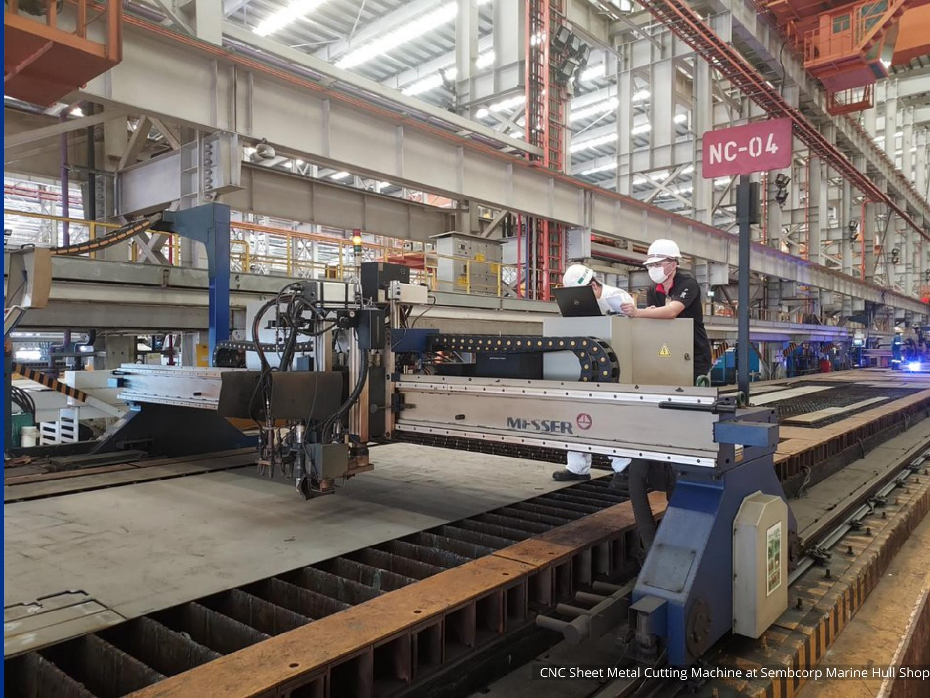
CNC Sheet Metal Cutting Machine at Sembcorp Marine Hull Shop
