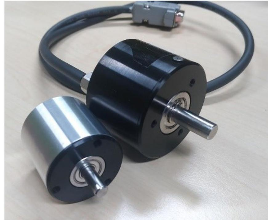
Low cost IP66 16-bit absolute magnetic encoder prototype
