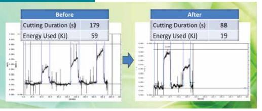
Optimised grinding wheels based on energy data analytics able to reduce the cutting time and energy consumption by 51 per cent and 68 per cent respectively.
