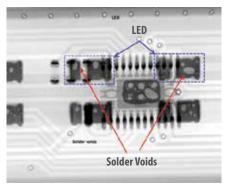
Figure 3: Bubbles of void due to inferior soldering during manufacturing
