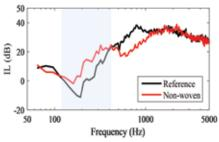
The comparison between the sound insertion loss (IL) of reference and non-woven flax fibre-reinforced PP earmuffs
