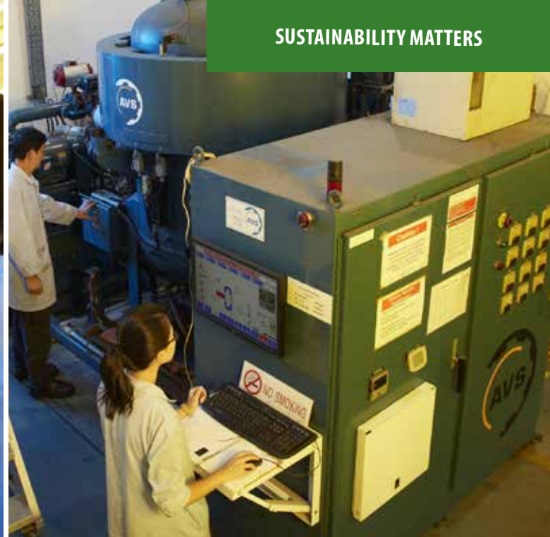
High temperature furnace for pure silicon carbide membrane sintering
