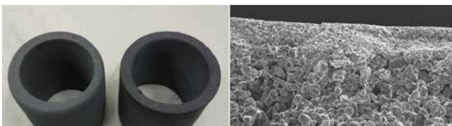
Pure silicon carbide membrane and microstructure
