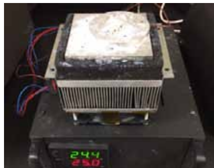
Figure 1: Peltier-based thermal performance analyser
