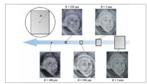
Scaling down of the machined grayscale images on metal surfaces
