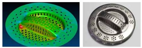
Figure 1: Development of metal "chokeless" strainer design and processing steps through simulation modelling (left) and stamping trials – a stainless steel strainer prototype with opening features optimised for stamping process steps (right)
