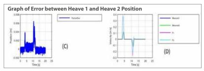
Figure 1 (A) The position(black) and command(blue) of hydraulic cylinder 1. (B) The position (black) and command(green) of hydraulic cylinder 2. (C) The position error between hydraulic cylinder 1 and hydraulic cylinder 2. (D) Measured velocity of hydraulic cylinder 1 and 2
