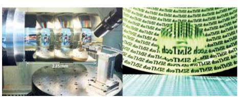
Machined linear/radial Fresnel lens roller moulds
