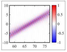
Snapshot of a non-diffracting laser beam with a tilted intensity profile. Axes are in micrometers
