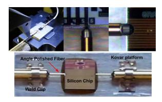
Lateral fiber assembly using laser welding technique: Fiber-to-fiber loss <8 dB, Excess loss <1.5 dB
