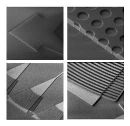
Silicon grating coupler: 2D grating to achieve polarisation diversity performance; Grating coupler with silicon overlay to reduce the coupling loss (<2.6 dB) on 220-nanometer (nm)-thick Silicon on Insulator (SOI)
