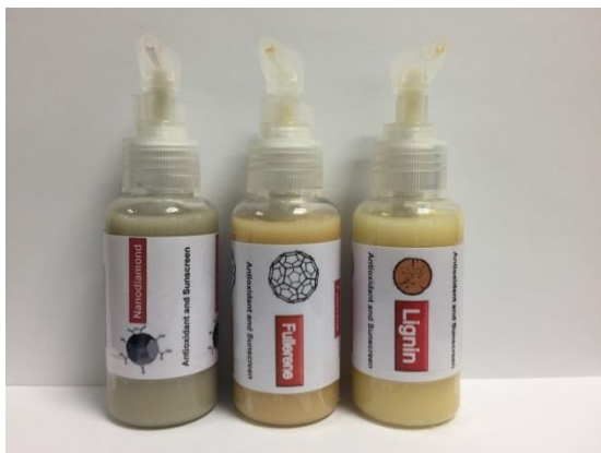
Prototypes of nanodiamonds (ND), fullerene ( C_{60} ) and lignin sunscreen. The colour intensity can be fine-tuned using different concentrations of ND, C_{60} and lignin.
