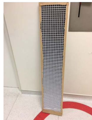
Prototype of IMRE-developed noise absorbing panel
