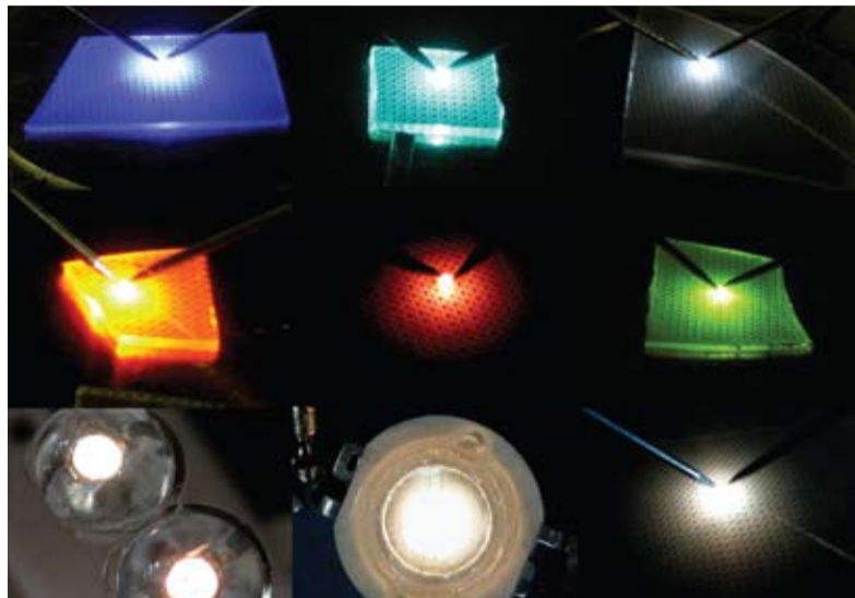
The coloured LEDs based on indium gallium nitride (InGaN) quantum wells (QWs) / quantum dots (QDs). The colour changes with the amount of indium in the materials. The improvement of InN material quality by capping will lead to high quantum efficiency for long-wavelength LEDs and make it possible to fabricate monolithic multi-coloured and white LEDs.
