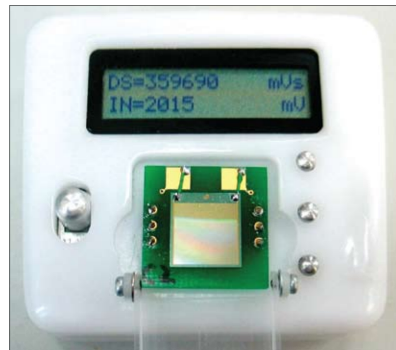
A prototype of the UV sensor
