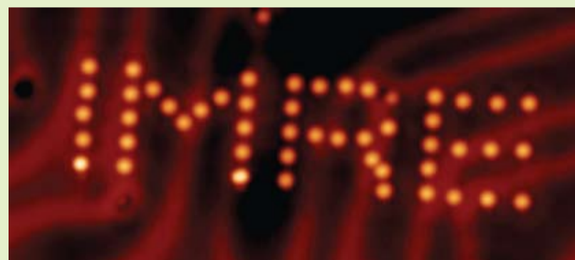
Scanning tunneling microscope image showing the word 'IMRE' formed by individual gold atoms
