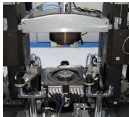
The nanoimprinter's top and bottom assembly allows a disk to be imprinted on both sides at one go
