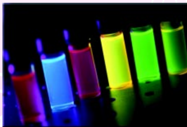
Short wavelength-emitting Zn_{1-x}Cd_xSe alloy nanocrystals excited with a UV lamp. The lab-on-a-bead technology allows more flexibility in target selection, faster binding kinetics and cheaper production.
