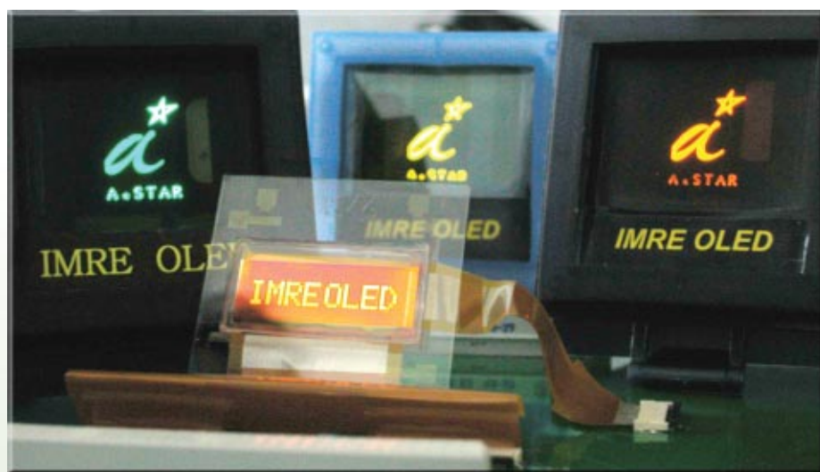
Prototypes of IMRE-fabricated OLED devices. (Front, centre) A polymer light-emitting passive matrix display surrounded by a number of different coloured OLEDs.
