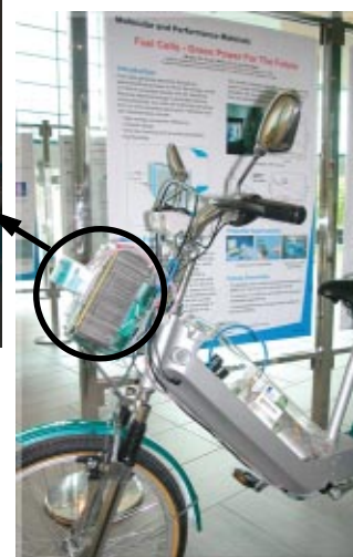
An IMRE fuel cell (above) fitted on the specially designed bicycle (right).
