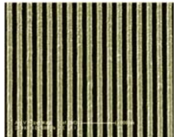
SEM image of aluminium grating with line width of 70nm used to generate polarised emissions from InGaN LED
