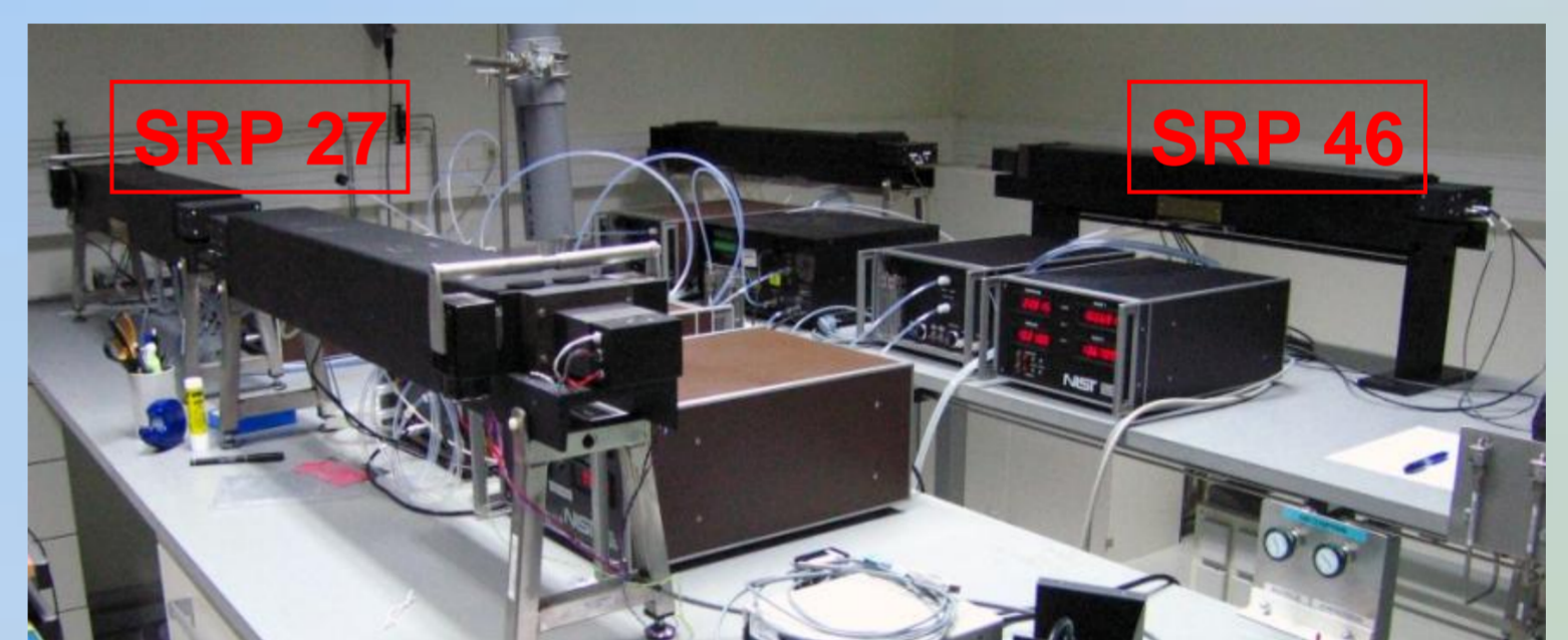
Comparison of NMC's Primary Ozone Standard SRP 46 with SRP 27 at the BIPM in France provides traceability in the measurement of ozone.
